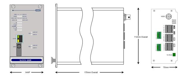
The **AMG5913-2A9R** is a rackmount one channel video transmit unit designed to transmit 1 video signal and transmit and receive 2 data signals, 2 audio channels plus 8 bi-directional alarms and also provides full duplex 100Base-T Ethernet connectivity over one Singlemode optical fibre.
